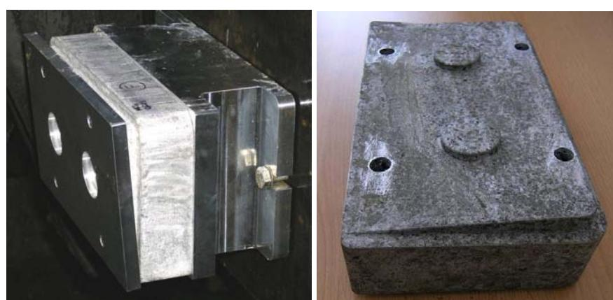
*Fig. 2. Assembled crash box of railway carriage containing Al foam (left) and Al foam component (right).*
