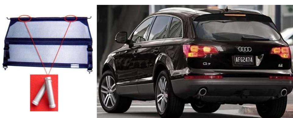
*Fig. 3. Aluminum foam crash energy absorber mounted into the dividing net of Audi Q7 developed by IMMM SAS.*
