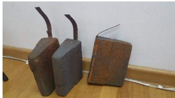
**Figure 3.1.** Y-blocks of ductile iron obtained from Split Shipyard
