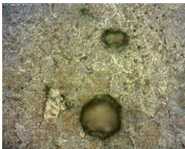
**Figure 4.6.** Austempered at 368°C without salt bath agitation, magnification 200x
