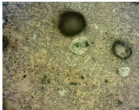
**Figure 4.2.** Austempered at 307°C with salt bath agitation, magnification 200x
