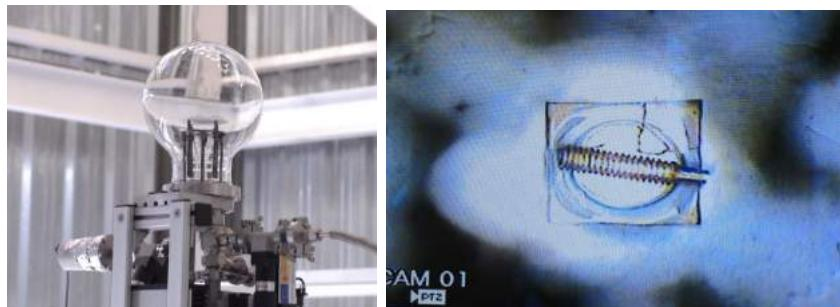
**Figure 3.** Vacuum/gas chamber used for gas nitriding (left) and sample with solar spot during experiment (right).
