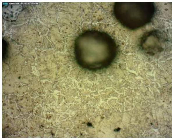
**Figure 4.5.** Austempered at 258°C without salt bath agitation, magnification 200x
