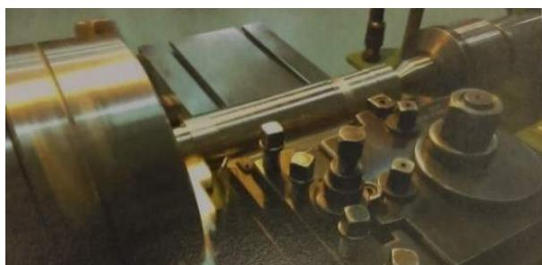
**Figure 1.** Turning of super duplex steel
