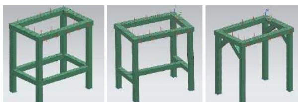
**Figure 3.** The body of the table divided into the finite number of simple shape elements
