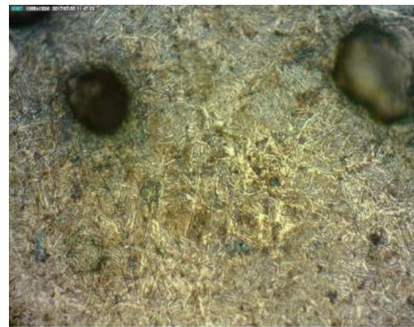
**Figure 4.7.** Austempered at 395°C without salt bath agitation, magnification 200x
