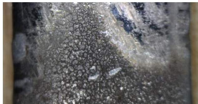
**Figure 2.** Thermal fatigue on the surface of H11 steel, [4]
