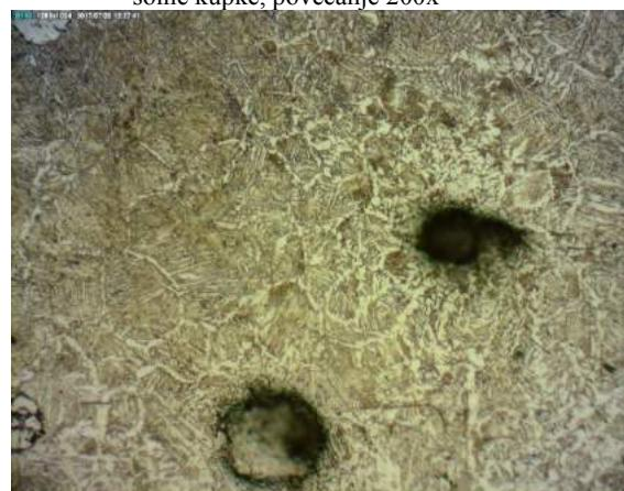
**Figure 4.4.** Austempered at 423°C with salt bath agitation, magnification 200x
