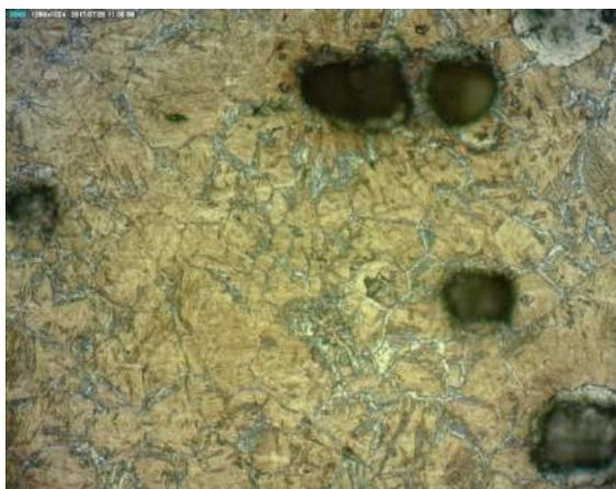
**Figure 4.1.** Austempered at 230°C with salt bath agitation, magnification 200x
