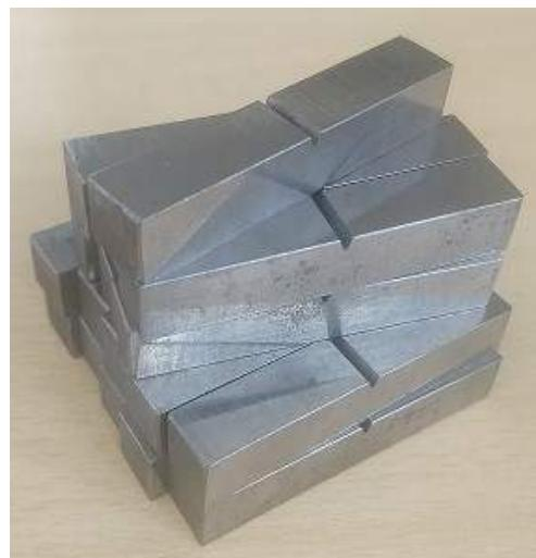
**Figure 3.2.** Standardized Charpy samples ready for experiments
