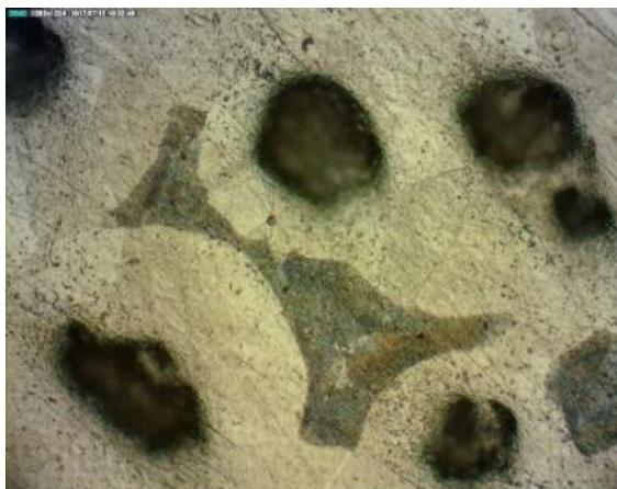
**Figure 3.3.** As cast microstructure, magnification 200x
