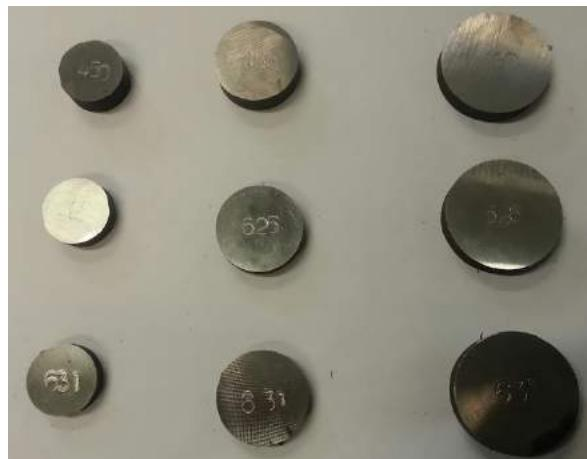
**Figure 5.** Specimens after heat treatment and cutting from the bar
