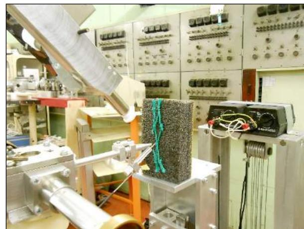
**Figure 4.** The fishing net sample 2 during the PIXE investigation.
