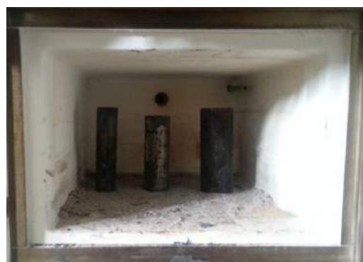
**Figure 3.** Bars of different diameter from which specimens were taken
