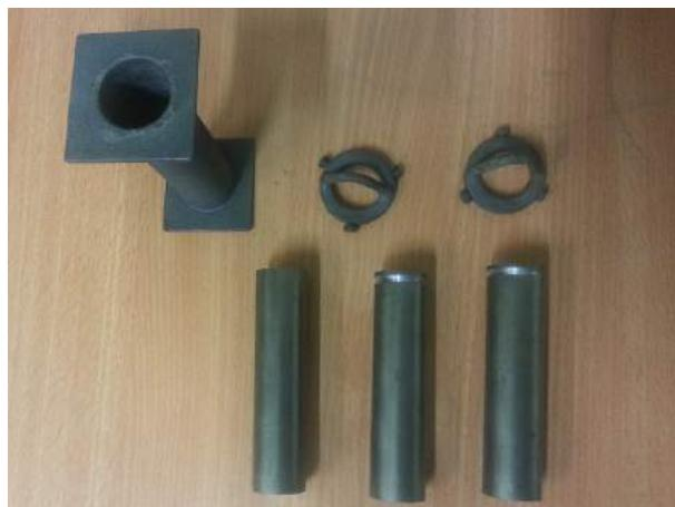
**Figure 4.** Jominy probes tempered at temperatures 450, 525 i 630°C
