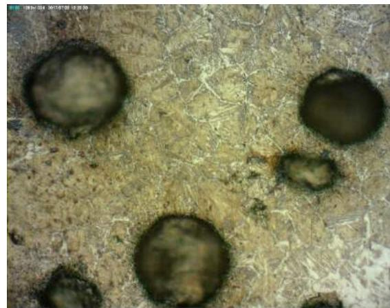
**Figure 4.3.** Austempered at 352°C with salt bath agitation, magnification 200x
