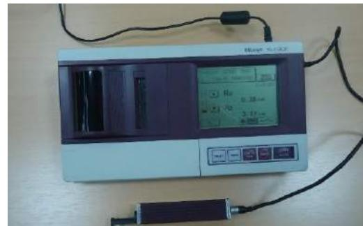
**Figure 2.** Surface roughness measuring device
