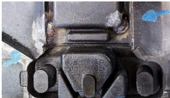
**Figure 3.** Mould surface repaired by TIG welding
